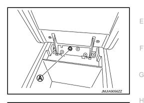
b. Pull back console rear finisher assembly, and then disengage metal clips according to the numerical order 1→2 as shown in the figure.
