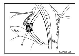
b. Pull instrument side finisher RH, and then disengage pawls using a remover tool (A) according to the numerical order 1→2 as shown in the figure.
