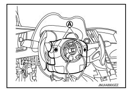
• Apply protective tape (A) on the part to protect it from damage.
