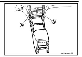
11. Remove the following part after removing center console assembly.
