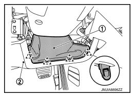
e. Disconnect harness fixing clips, and then remove harness connectors and aspirator duct.
