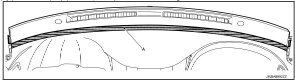
Disengage front speaker grille fixing metal clips starting from both sides and work toward the center of the front speaker grille as 1→2 as shown in the figure.
