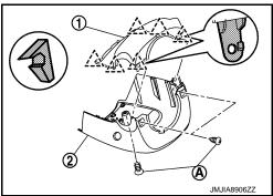
• Disengage pawls of cluster lid A apron portion ② and remove steering column upper cover ①.
