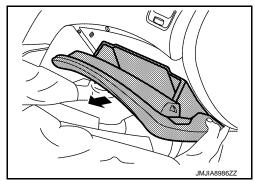
c. Pull glove box assembly damper string and remove it from glove box assembly ①.
