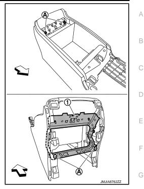
3. Disengage center console finisher fixing pawls and remove center console finisher.
