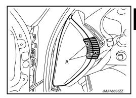
b. Pull instrument side finisher LH, and then disengage pawls using a remover tool (A) according to the numerical order  $1{\to}2$  as shown in the figure.
